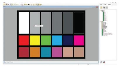
It is recommended to perform the White Balance after a CSR and on a white or gray object that is not fully saturated.
